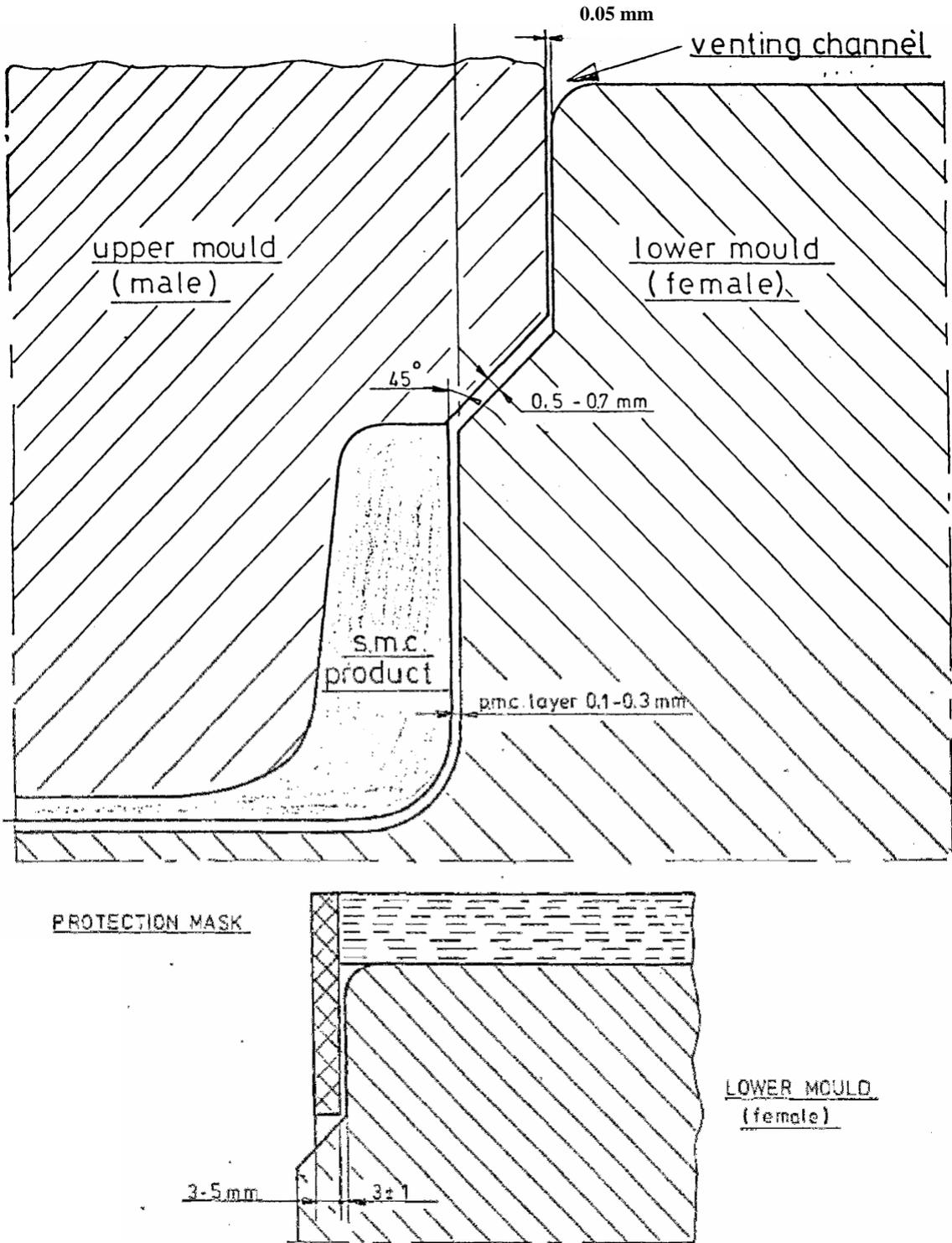
Figure 3: Preferred mould venting design.
