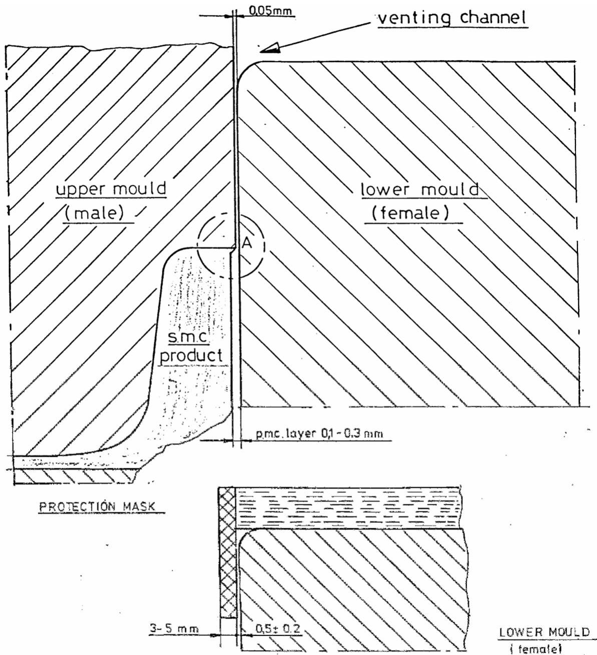
A - At this point of the mould the PMClayer is being destroyed and the venting channel will be blocked, causing possible blisters on the part
